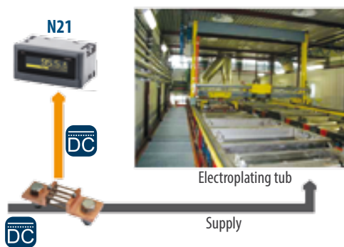
Current measurement in an electroplating plant
